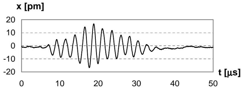
**Figure 6:** Averaged surface displacement response on exciting signal from figure 4.
