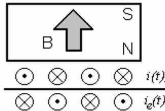
**Figure 1:** Principle of Rayleigh EMAT type.
